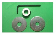
We are going to epoxy the 2 - 1 1/2" washers to the 3/8" collar. This will become the base for the Image light or any other portable light that you can direct the light on to the fly you are tying. Light is always an issue when you are tying away from home.
