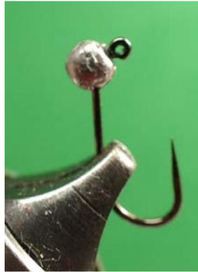
A coat of powder paint will make up the lost. So if I powder paint my 1/100th, and if I made a mold, I will get Jiglopy of 1/100th. So if I powder paint my jiglopy with 3 to 4 coats of powder paint, I will get to the 1/80<sup>th</sup> size. If I powder paint my jiglopy with 5 to 6 coats, I will get to the 1/64<sup>th</sup> size.
