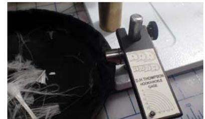
Cut a 3 inch pin out the extra 3/8" rod and attach a waste basket and a hackle gauge.
