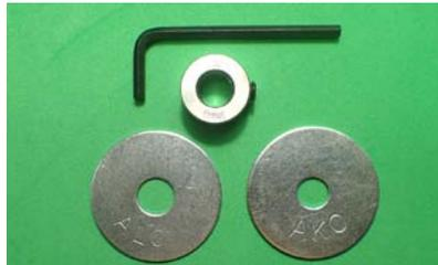
We are going to epoxy the 2 - 1 1/2" washers to the 3/8" collar. This will become the base for the Image light or any other portable light that you can direct the light on to the fly you are tying. Light is always an issue when you are tying away from home.
