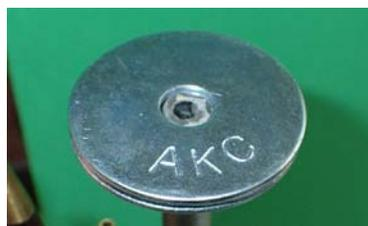
Drill a hole in the top of the rod to fit the wire of a parachute hanger. Then when you need it, remove the light and add the hanger
