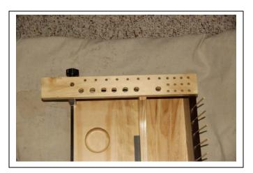
The tool holder shelf measures 2" x 14 3/8" and all the wood used is .750 thick.
